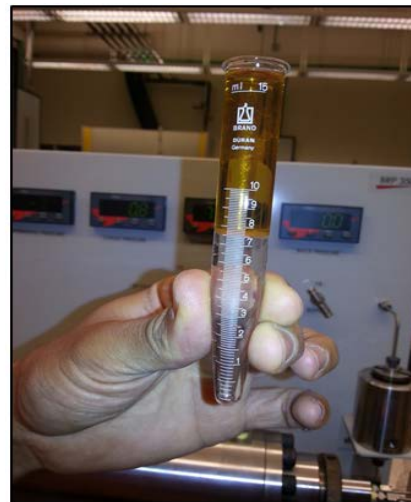
Figures 7 and 8. Oil displacing water to measure S_{wi} (left); total displaced water volume (right).
